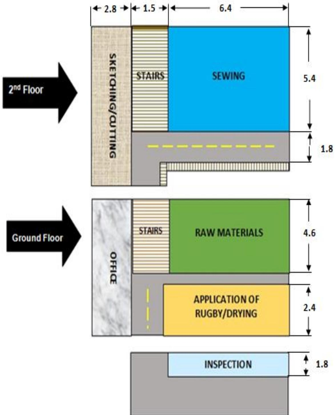
Figure 4. Current Production Layout for Insole and Tope (Location B)
