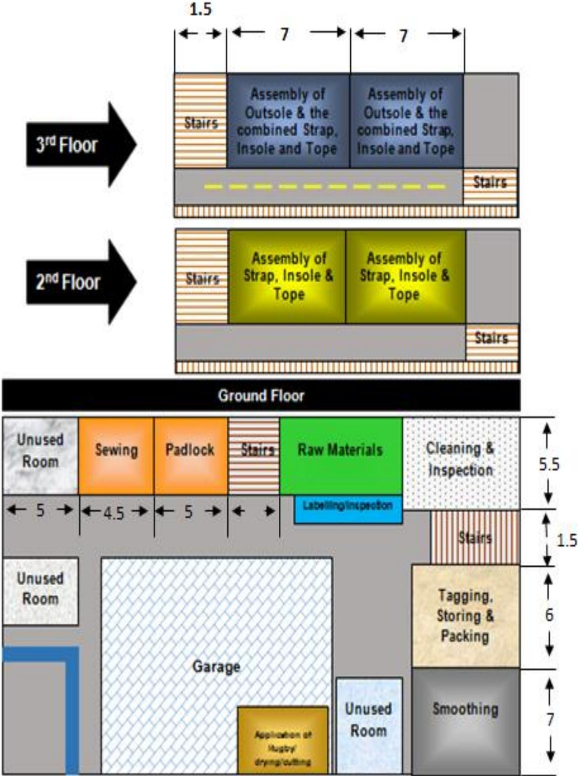
**Figure 5.** Current Production Layout for Outsole (Location C)
